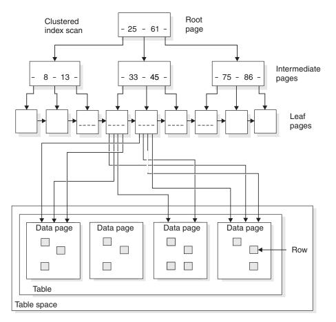
*Figure 35. A nonclustered index scan.* In some cases, DB2 can access the data pages in order even when a nonclustered index is used.
