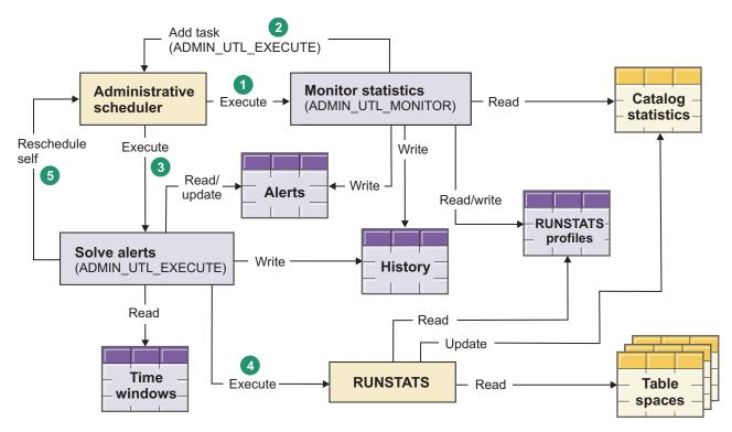
Figure 33. Object interactions for autonomic statistics maintenance in DB2
