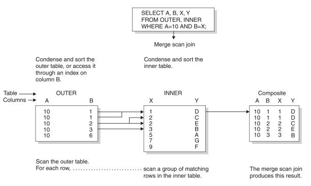
Figure 52. Merge scan join
