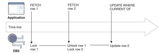
Figure 16. Positioned updates and deletes with a static non-scrollable cursor and without optimistic concurrency control
