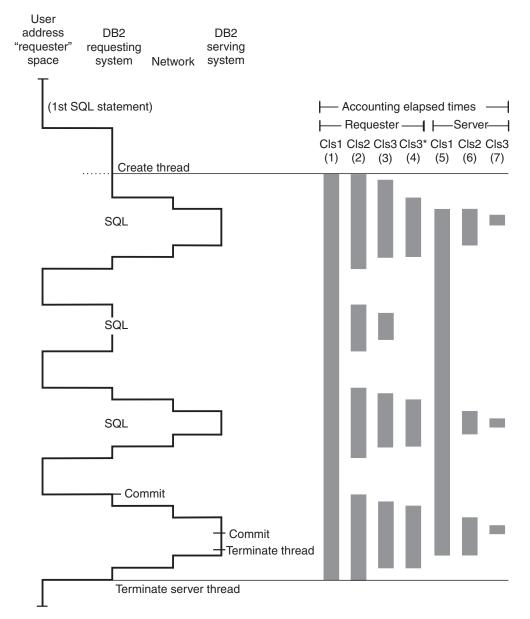
*Figure 45. Elapsed times in a DDF environment as reported by OMEGAMON.* These times are valid for access that uses DRDA(except as noted).
