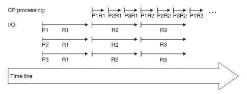
Figure 29. CP and I/O processing techniques. Parallel I/O processing.
