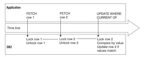
Figure 17. Positioned updates and deletes with a static sensitive scrollable cursor and with optimistic concurrency control
