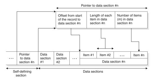
Figure 64. Relationship between self-defining section and data sections for same-length data items
