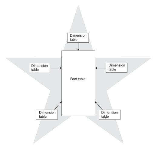
Figure 54. Star schema with a fact table and dimension tables
