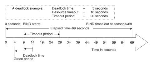
Figure 2. An example of scanning for timeout
