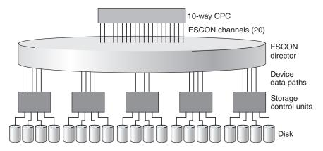
Figure 31. I/O configuration that maximizes performance for an I/O-intensive query
