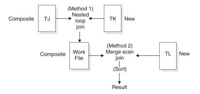
Figure 50. Two-step join operation
