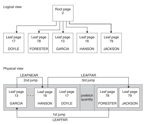
Figure 32. Logical and physical views of an index in which LEAFNEAR=1 and LEAFFAR=2
