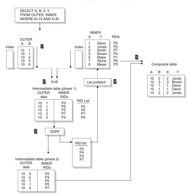
Figure 53. Hybrid join (SORTN\_JOIN='Y')
