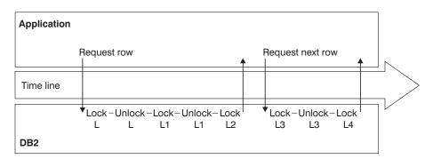
*Figure 18. How an application that uses RS isolation acquires locks when no lock avoidance techniques are used.* Locks L2 and L4 are held until the application commits. The other locks aren't held.
