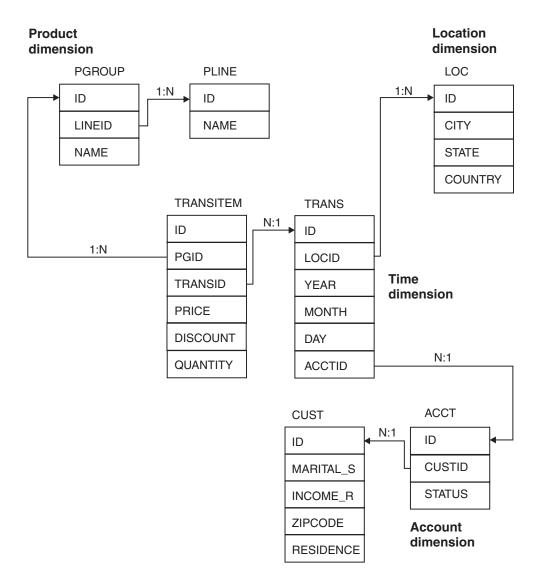
*Figure 15. Multi-fact star schema.* In this simplified credit card application, the fact tables TRANSITEM and TRANS form the hub of the star schema. The schema also contains four dimensions: product, location, account, and time.
