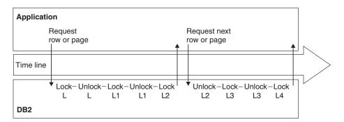
Figure 19. How an application that uses CS isolation with CURRENTDATA (YES) acquires locks. The figure shows access to the base table. The L2 and L4 locks are released after DB2 moves to the next row or page. When the application commits, the last lock is released.
