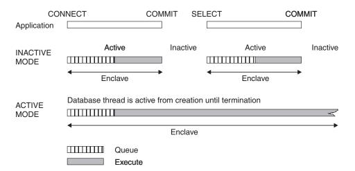
Figure 46. Contrasting ACTIVE MODE threads and POOLED MODE threads
