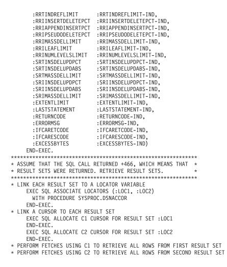
Figure 79. Example of DSNACCOR invocation
