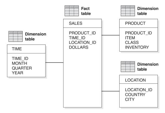
Figure 55. Example star schema with 3 dimension tables
