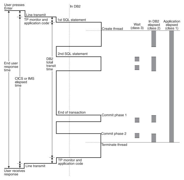
*Figure 47. Transaction response times.* Class 1 elapsed time includes application and DB2 elapsed times. Class 2 elapsed is the elapsed time in DB2. Class 3 is elapsed wait time in DB2. Standard accounting data is provided in IFCID 0003, which is turned on with accounting class 1. When accounting classes 2 and 3 are turned on as well, IFCID 0003 contains additional information about DB2 CPU times and suspension times.
