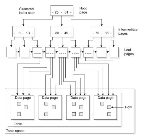
Figure 34. A clustered index scan. This figure assumes that the index is 100% clustered.
