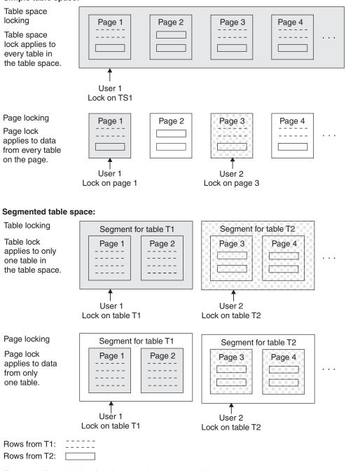
Figure 13. Page locking for simple and segmented table spaces
