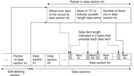
Figure 65. Relationship between self-defining section and data sections for variable-length data items
