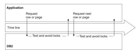
Figure 20. Best case of avoiding locks by using the ISOLATION(CS) and CURRENTDATA(NO) options. This figure shows access to the base table. If DB2 must take a lock, locks are released when DB2 moves to the next row or page, or when the application commits. This behavior matches the CURRENTDATA(YES) option.
