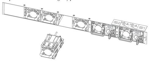
**Attention:** If the inlet air temperature is above 35°C (95°F) while the switch is in operation, replace the fan module within five minutes to avoid overheating the switch.
