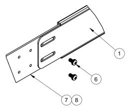
4. Loosen and remove the M6 screws, washers, and clip nuts (or cage nuts) that attach the filler plate and rear mounting brackets to the rear rack posts.
