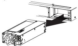
**Attention:** Do not leave the power-supply bay empty for more than 90 seconds while the switch is operating. Either replace the power supply module or install a blank power filler plate.
