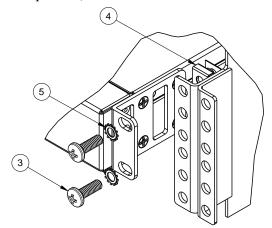
6. Attach the rear alignment plate (Item 7) to the rear rack posts with M6 screws (Item 3), washers (Item 5), and clip nuts (Item 4). Torque the screws to approximately 5.7 Nm +/- 0.1 Nm (50 inch-pounds).
