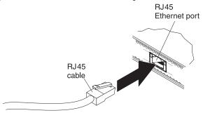
To disconnect the RJ45 cable, squeeze the release tab and gently pull the cable connector out of the switch connector.
