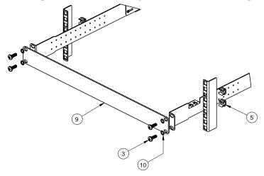
5. Slide the rear mounting brackets out of their slots in the front mounting brackets.
