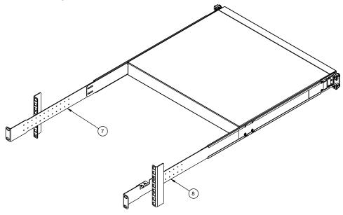
7. Attach the filler plate (Item 9) and rear mounting brackets to the rear rack posts with M6 screws (Item 3), washers (Item 10), and either clip nuts (Item 4) or cage nuts (Item 5). Torque the screws to approximately  $5.7 \text{ Nm} \pm 0.1 \text{ Nm}$  (50 inch-pounds).
