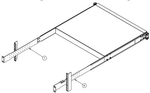
6. Loosen and remove the M6 screws, washers, and clip nuts (or cage nuts) connecting the front mounting brackets to the front rack posts.
