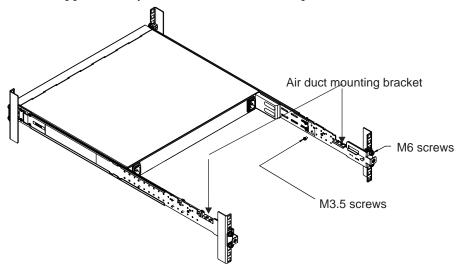
**Note:** Reuse the original M6 screws used to fasten the 4-post rack mounting brackets to secure the air duct mounting brackets with 4-post mounting brackets together.
