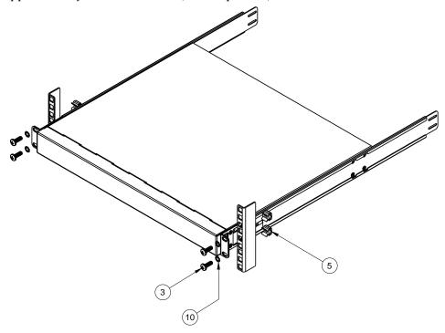
6. Slide the rear mounting brackets (Item 7 and Item 8) into the slots available on the front mounting brackets.
