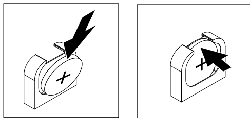
Figure 204. Coin-cell battery installation
