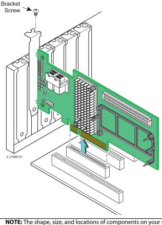
**NOTE:** The shape, size, and locations of components on your controller and its bracket might vary from this illustration. The controller requires an x8 PCIe slot.
